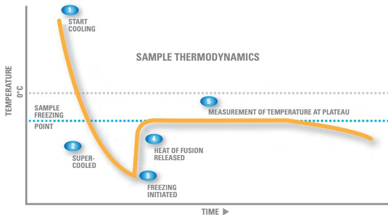
Advanced osmometers utilize the industry-preferred freezing point depression method to determine the osmolality of an aqueous-based solution. When a solute (particles) is dissolved in a solvent (water), the freezing point of that solution is lowered compared to that of the solvent alone. As more solute is added, the freezing point decreases further. Therefore, by precisely measuring the freezing point of the solution, the osmolality (i.e., concentration) can be determined.
